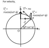
The velocity projection on y axis will be  $v_y = v \cos\theta = r\omega \cos\theta$  $= r\omega \cos(\omega t + \varphi)$
