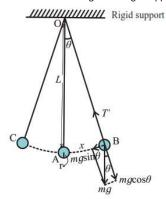
L: distance from the suspension and centre of gravity of the bob (length of pendulum) m: mass of the bob T' : Tension in the string at extreme position  $\theta$ : Small angle the pendulum is displaced by and then released A: mean position
